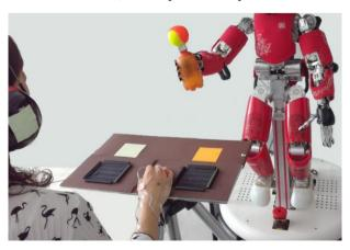
Figure 2. Experimental Setup included the working table with two target areas (yellow and orange) and the humanoid robot iCub standing in front of the subject. The face of the robot was covered to avoid bias regarding eyes or facial information.
