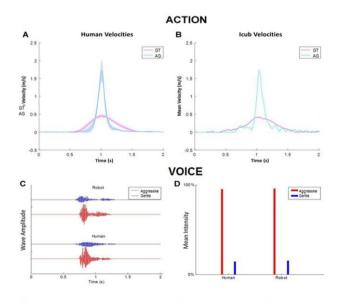
Figure 5. Action: velocity profiles of the movements performed by the human actor (A) by robot (B). Voice: graphs show the wave amplitude (C) and the mean intensity (D) relative to the action verb "take it" pronounced by human and iCub robot in gentle and rude way.
